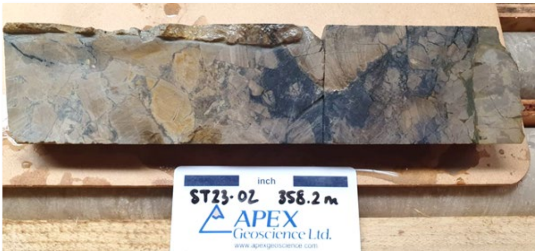
Figure 1: Photo of strong chalcocite (dark grey) breccia fill and veining in drill hole ST23-02 from approximately 358.2m downhole. Chalcocite is a copper sulfide mineral and contains approximately 79.8% copper.
